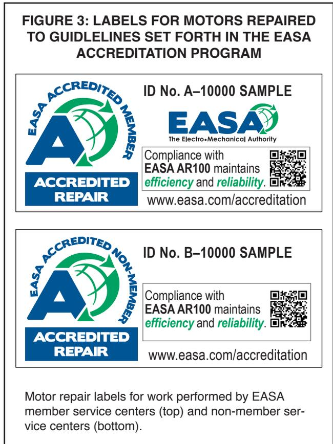
Electric motors that conform to the requirements of the criteria in the associated checklists are to be labeled by the service center with an EASA label (Figure 3). Conversely, motors that do not meet the requirements cannot be labeled. The labels will be available for purchase by accredited service centers in quantities of 100 from EASA.
